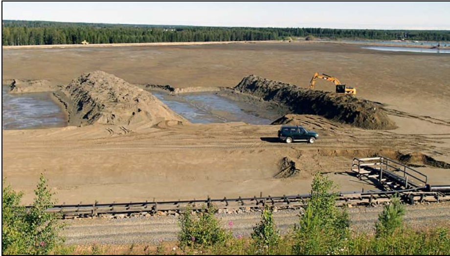
Figure 6.7. Stacking of pyrite in Pond B in summer 2012, Pyhäsalmi Mine Oy Photo: H. Karjalainen
