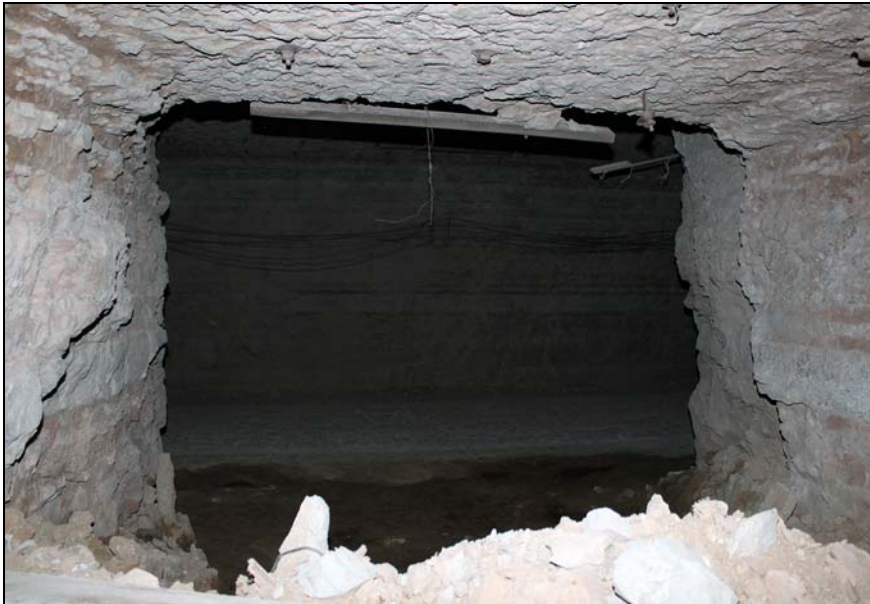
Figure 6.14. Room and pillar mining in Estonian oil shale mine Source: Tallinn University of Technology, Department of Mining
