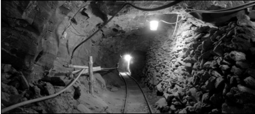
Figure 6.26. One of the old headings planned for liquidation using dry flooring at the Bochnia Salt Mine; Bochnia, Poland
