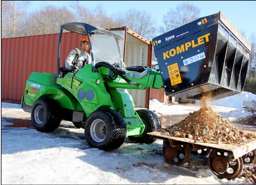
Figure 3.9. Mini wheel-loader equipped with crushing bucket Photo: Tallinn University of Technology
